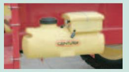
Century's optional **foam marker** provides 14-gallon capacity, dual drop bells and in-cab control console.
