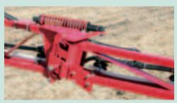
Eleven-foot outer wing is protected by a self-returning, shock absorber dampened breakaway system.
