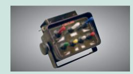
All boom functions are **hydraulically controlled** from the in-cab console. Boom lift, lower, wing tilt and fold functions require only one tractor remote.
