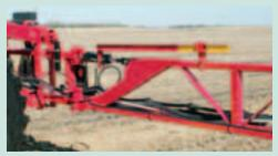
**Hydraulic accumulators** are provided on main and wing lift cylinders to provide shock cushioning and are combined with spring centered, self-leveling linkage to assure a smooth boom ride.
