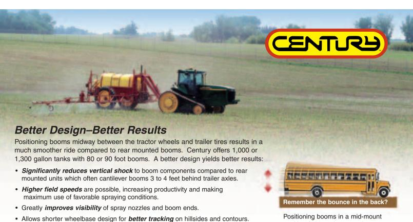
position (midway between the tractor wheels and trailer wheels) results in a much smoother ride compared to rear mounted booms which are often positioned 3-4 feet behind the trailer axle.
