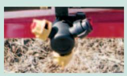
Non-drip, **triple nozzles** on 20" spacing are provided as standard equipment. Tip selection is accomplished with just a twist. Boom clamps are stainless steel. An adjustable auxiliary spray nozzle is located behind each Trailer Tire.
