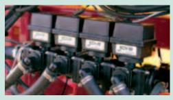
Boom on/off functions are controlled by 300 psi **motorized ball valves** for long life and high flow capacity. (4) on 80 ft. or (5) on 90 ft.
