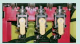
Conveniently located **control manifold** provides easy access control of agitation, bypass and rinse functions. Flanged fittings are used where possible.
